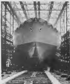
FRICION FROM the weight of the tremendous Esso tanker sets the special launching lubricants to smoking as the Esso Aruba slips into the harbor.
